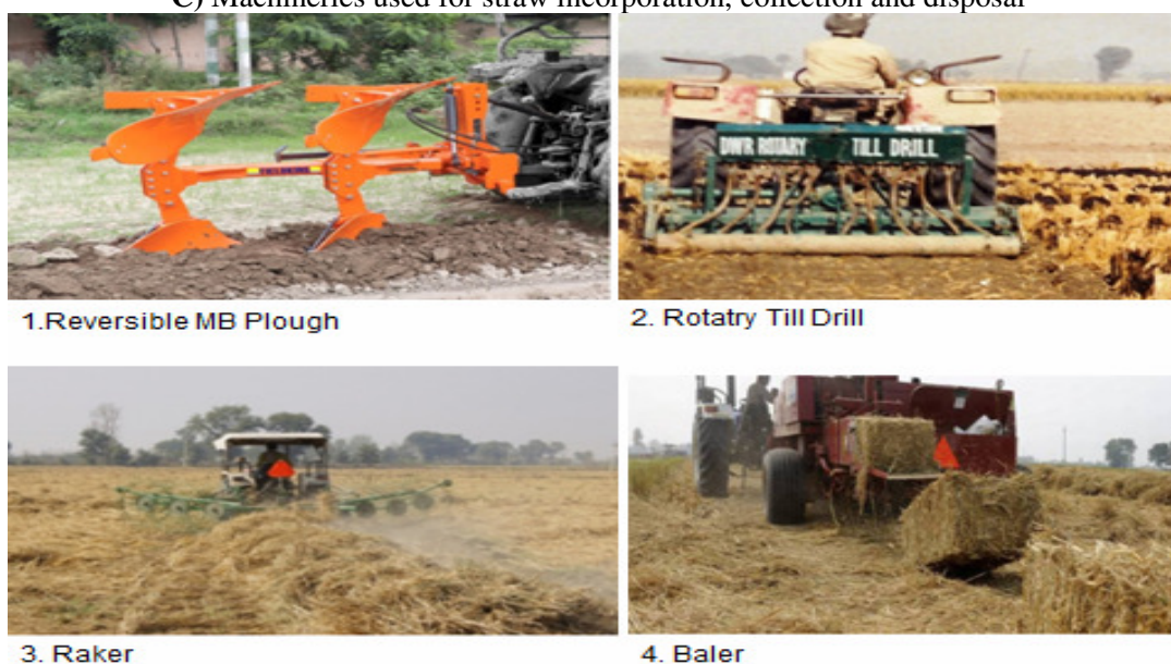
Fig. 3 : Machineries used for sowing crop under paddy residue.
